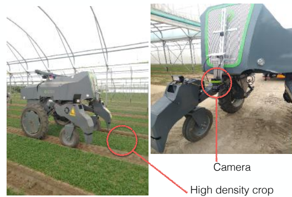
Figure 1. Global view of the imaging system fixed on a robot moving above mache salads of high density. RGB images are captured by a JAI manufactured camera of 20 M pixels with a spatial resolution of 5120 \times 3840 pixels, mounted with a 35 mm objective. The typical distance of plants to camera is of 1 m.
