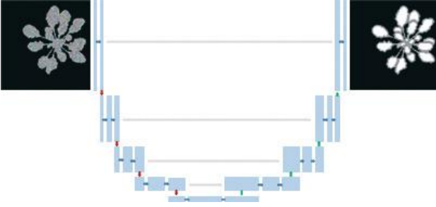
Figure 1: U-Net architecture. Each blue box corresponds to a multi-channel feature map. Gray arrows indicate the merging of the context and localization information that was done by concatenating the features from the contracting path with the corresponding ones in the expansion path. Input image has 128x128 pixels, the output of the model is a three-channel binary image: mask without contours, leaf contours and background.
