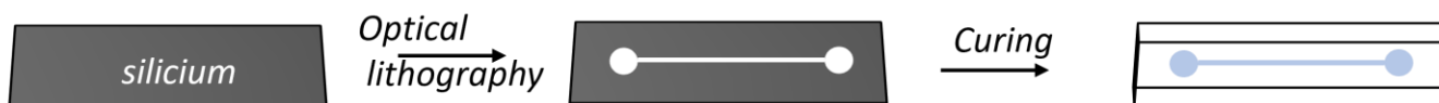
Figure 2. Microfabrication key steps: inverted optical lithography, Ti/Au metallization, PDMS fabrication and bounding (not shown here).
