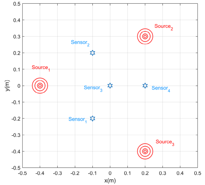
FIGURE 1 Positions of the plate’s 3 sources and 4 sensors.
