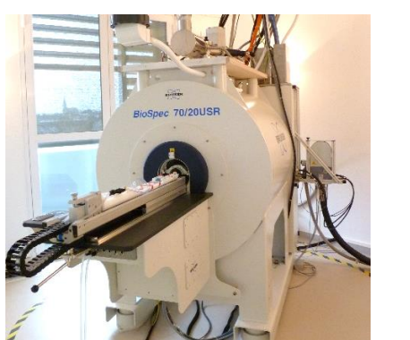
Imageur 7T Angers (Bruker BioSpec 70/20)
