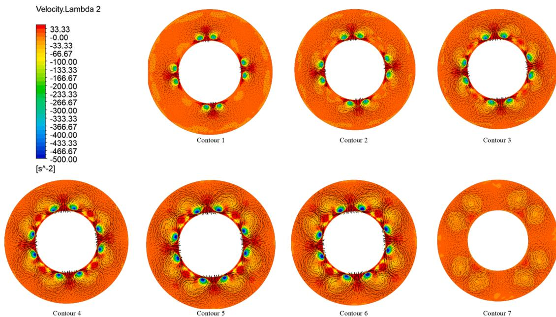
Fig. 12. Vorticity profiles of case 2 for  $Re_{hw}=8000 - Re_{cw}=2000$ .
