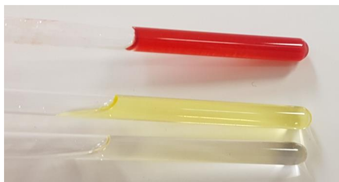
Figure 2. Top. Donor-acceptor organogel obtained from C 3 NDI and C 3 Pyr in TCE-d 2 ([C 3 Pyr] = [C 3 NDI] = 5.2 mM). Middle. Solution of C 3 NDI in TCE (5.2 mM). Bottom. Solution of C 3 Pyr in TCE (5.2 mM).
