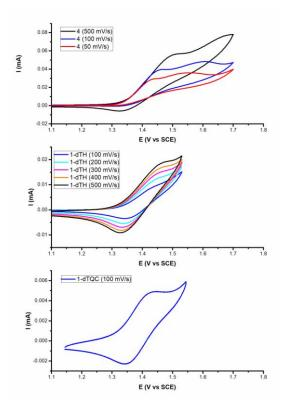
Figure 2. Cyclic voltammetry of 4 (1.24 mM), 1-dTH (1.24 mM) and 1-dTQC (1.04 mM) using  $TBAPF_6$  electrolyte (100 mM solution in dichloromethane) at different scan rates.
