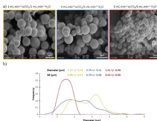
**Fig. 4.** Impact of the total flow rate on the microfluidic process. Conditions: 40°C, same flow rate for the scCO<sub>2</sub> and the aqueous calcium chloride solution, coflow micromixer, P = 250 bar, without polymer. a) Representative scanning electron microscopy (SEM) images of the CaCO<sub>3</sub> particles from left to right (yellow, blue, red): 1, 3 and 6 mL/min for each phase, b) particle diameter distribution determined from several SEM images: 1-, 3- and 6- mL/min for each phase.
