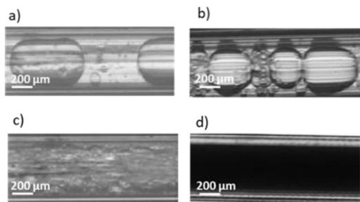
Fig. 2. Representative light microscopy images of the different observed dispersion states within the microfluidic channel no matter the operating conditions. a) slugs; b) extremely large droplets; c) smaller droplets; d) droplets so small that they are not distinguished by the camera (very efficient dispersion). The conditions leading to these different dispersion states are detailed in the different sections, highlighting the role of each parameter ( $P$ , flow
