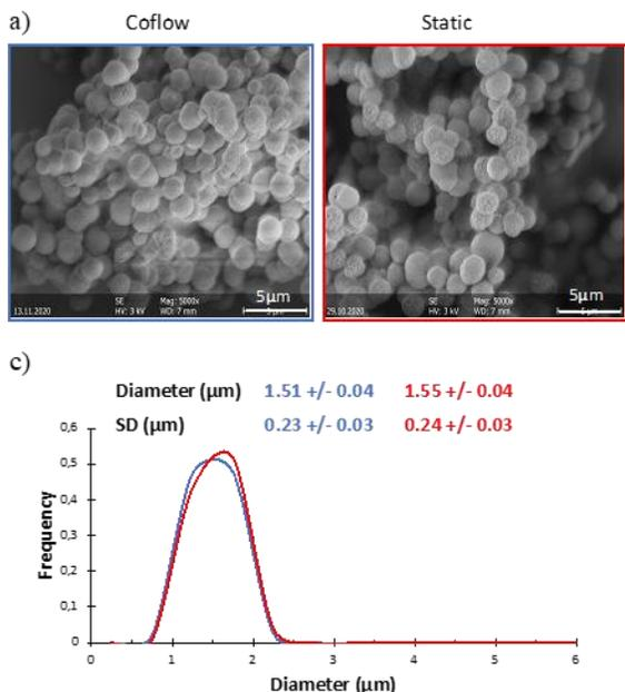
Fig. 5. Impact of the type of micromixer. Conditions: 40°C, 6 mL/min of  $\text{scCO}_2$  and 6 mL/min of aqueous calcium chloride solution,  $P = 250$  bar, different micromixers: Left (blue): coflow micromixer, Right (red): static micromixer. a) Representative scanning electron microscopy (SEM) images of the  $\text{CaCO}_3$  particles, b) particle diameter distribution determined from several SEM images.
