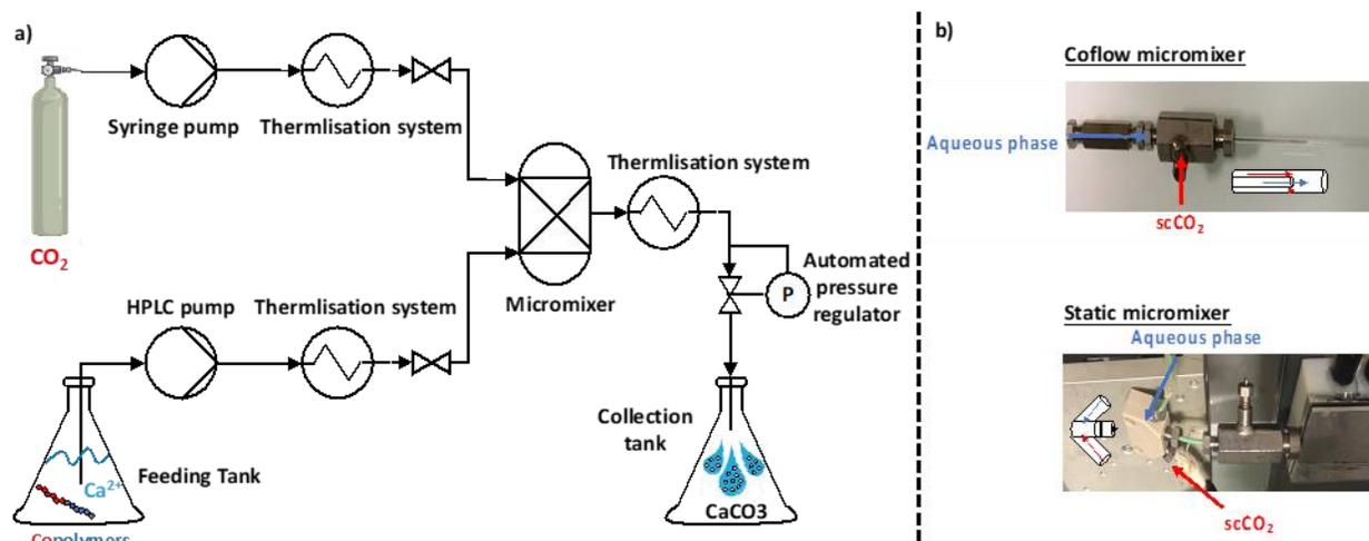
Fig. 1. a) Microfluidic pilot setup equipped with a micromixer for the continuous formulation of  $\text{CaCO}_3$  microparticles in  $\text{scCO}_2$ -water dispersion with b) a coflow or a static micromixer.
