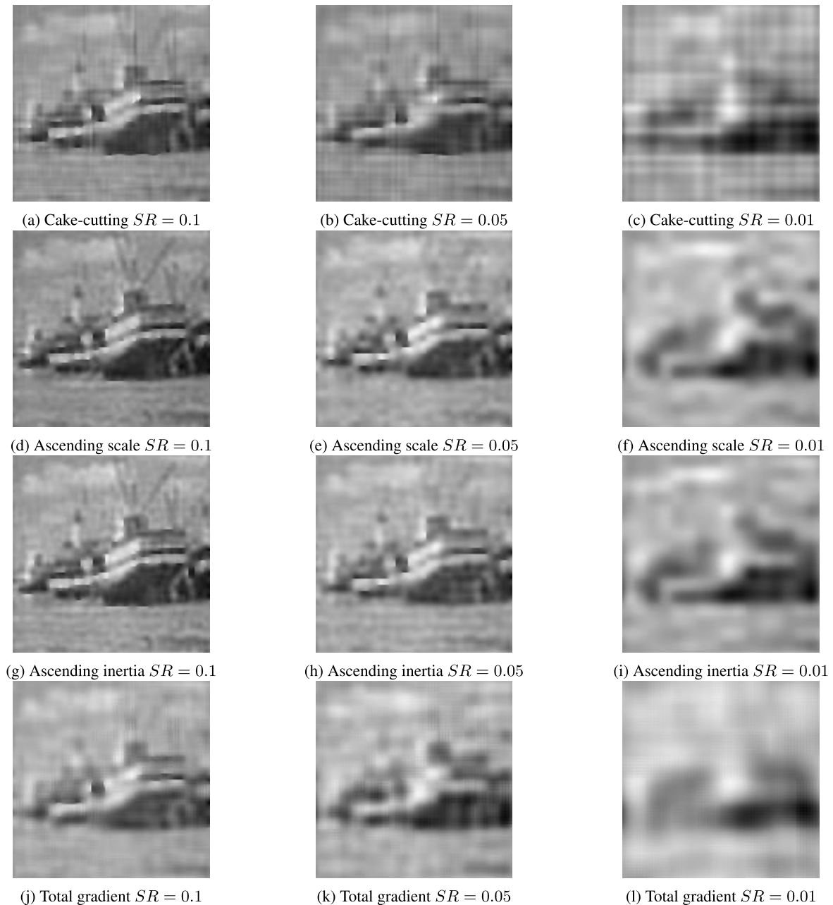
FIGURE 4. Image reconstruction of boat using TVAL3 algorithm for the simulation with a noise level of c = 0.1 .
