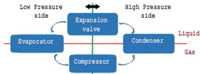
Figure 1. Refrigeration cycle basic working process [26].
