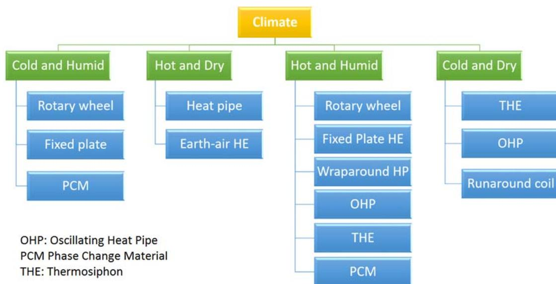
Figure 6. Heat recovery devices according to the climate.
