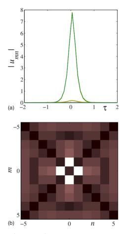
FIG. 10. (Color online) An example of a stable quadrupole soliton, which self-traps form initial configuration (27) with  $\mu$ =25 (the quadrupoles are stable for  $\mu \ge 20$ ). The panels have the same meaning as in Fig. 1 [the top panel displays the field profiles at the lattice sites belonging to "frame" (5), and in the next layer, formed by the sites with |m|=2, n=0 and m=0, |n|=2].
