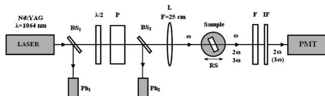
FIG. 1. Experimental setup for SHG and THG measurements: the beam splitters (BS<sub>1</sub>, BS<sub>2</sub>), the synchronization and control photodiodes (Ph<sub>1</sub>, Ph<sub>2</sub>), ( $\lambda/2$ ), the Glan polarizer, the converging lens, RS, the filters, IF, and PMT.
