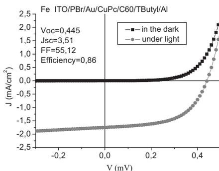
**Figure 4.** J-V curves of a solar cell using PTBrPDSe as “buffer layer” Glass/ITO/PTBrPDSe/Au/CuPc/C<sub>60</sub>/Tbut/Al.
