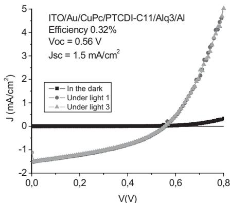
**Figure 2.** J-V curves of a solar cell using PTCDI-C11 as acceptor layer. Glass/ITO/Au/CuPc/PTCDI-11/Alq<sub>3</sub>/Al.
