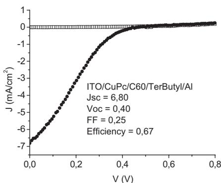
**Figure 3.** J-V curves of a solar cell Glass/ITO/CuPc/C<sub>60</sub>/Tbut/Al.
