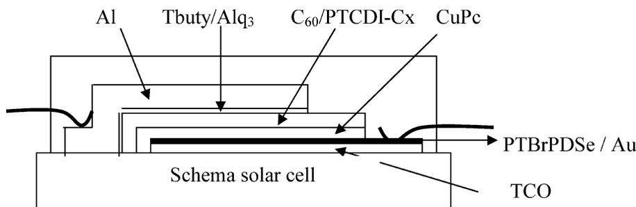
For PV-cells, organic materials were purified by vacuum sublimation. Besides, it was observed that using the same charge in the evaporation crucible led to “self-purification” of the product during the first depositions. Therefore, the results discussed herein correspond to cells deposited after at least five evaporation cycles of the organic products.
