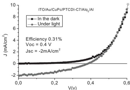
**Figure 1.** J-V curves of a solar cell using PTCDI-C7 as acceptor layer. Glass/ITO/Au/CuPc/PTCDI-C7/Alq<sub>3</sub>/Al.
