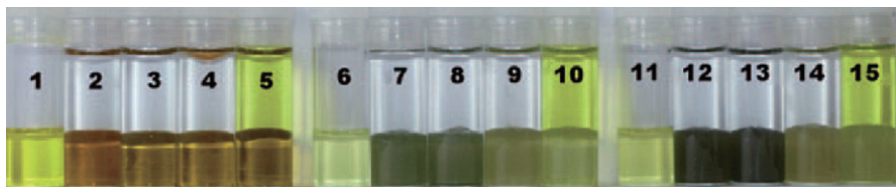
Figure 9.11. Visual color changes induced by the addition of 2 mL of 0.1 mM solutions of 22 , 31 , and 32 in \text{CHCl}_3 to 3 mL of 0.2 mM aqueous solutions of the test nitroaromatic explosives TNB, PA, and TNT in the absence and presence of salts [30]. Here, “salts” refer to a mixture of \text{NaHCO}_3 , \text{K}_2\text{CO}_3 , \text{MgSO}_4 , \text{CaCl}_2 , and \text{NH}_4\text{Cl} , 2 mM in each experiment. The contents of the vials from left to right are as follows: (1) pure 22 , (2) 22 + TNB, (3) 22 + TNB + salts, (4) 22 + TNT, (5) 22 + PA, (6) pure 31 , (7) 31 + TNB, (8) 31 + TNB + salts, (9) 31 + TNT, (10) 31 + PA, (11) pure 32 , (12) 32 + TNB, (13) 32 + TNB + salts, (14) 32 + TNT, and (15) 32 + PA. Source: [30]. Reproduced with permission of Wiley-VCH Verlag GmbH & Co. KGaA. See color insert.
