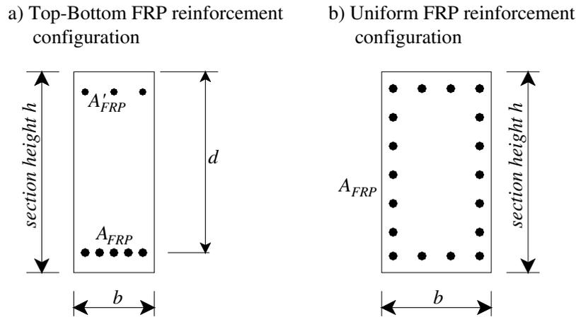
**Figure 3. Top-Bottom and Uniform FRP reinforcement configuration.**
