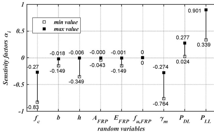
**Figure 11. Maximum and minimum values of sensitivity factors  $\alpha_i$  of random variables considered (Uniform configuration).**
