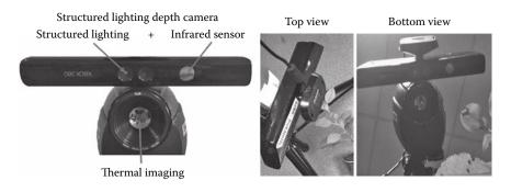
*Figure 9.9* (See color insert.) Left: The anatomofunctional imaging system in this chapter is composed of a depth camera using the 2D structured lighting (binary dot pseudorandom grid) method and a thermal imaging. Right: An acquisition on a plant is done by one shot taken in plant top view.
