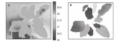
*Figure 9.11* (See color insert.) An anatomofunctional imaging composed of depth camera and a functional imaging allows us to have two registered images: the depth map and the functional image. In this chapter, the anatomofunctional imaging system is composed of (a) a thermal imaging providing a thermal image and (b) a depth camera providing a depth map.
