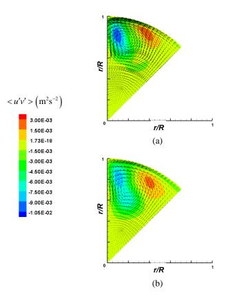
Figure 2. Reynolds shear stress distribution on two cross sections located at (a) z/h=0.75 and (b) z/h=2.5 downstream from the tab, Re=15000
