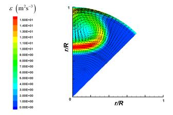
Figure 5. Distribution of the turbulent energy dissipation rate computed on a cross section located at z/h=0.75 downstream from the tabs, for Re=15000
