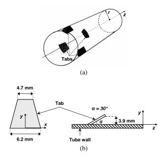
Figure 1. (a) Global view of the test section and (b) mixing tab dimensions
