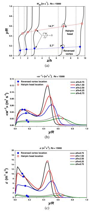
Figure 3. Experimental radial profiles of the (a) mean streamwise velocity, (b) Reynolds shear stress  $\langle w'^2 \rangle$  and (c) turbulent energy dissipation rate, showing the development of primary hairpin heads (O) and reversed vortices ( $\bullet$ ) for z/h = 0.75 to 8.75 downstream from the tab, *Re*= 15000.
