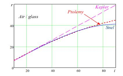
$\rightarrow$  In all three cases up to 70°, the experimental "measurements" seem close to the values given by Snell's law
