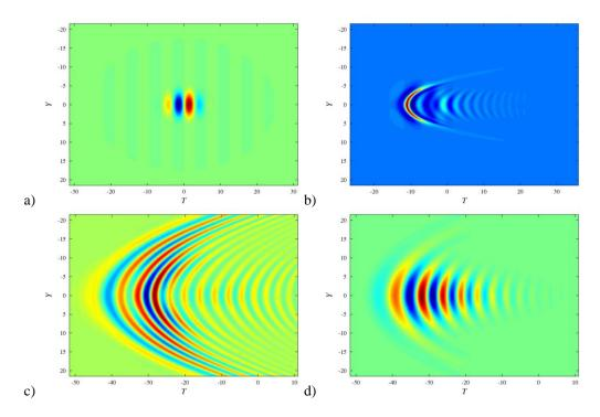
**Figure 1** Nonlinear diffraction of the FCP: (a) input profile at the (*y*, *t*)-plane; (b) an intermediate stage with a typical crescent shape; (c) nonlinear diffraction; (d) linear diffraction.
