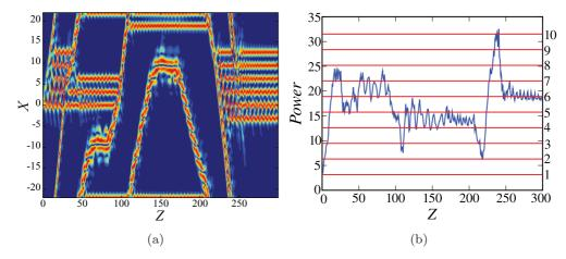
FIG. 19. (Color online) (a) Example of the complex interaction of the free soliton with the standing structure at  $k_0 = 1.693$  and  $\theta = 0$ . (a) Distribution of the field |u(X,Z)| in the cross section Y = 0 and (b) total power versus Z. In panel (b) horizontal lines show the multiple powers of the quiescent fundamental soliton.
