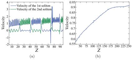
FIG. 20. (Color online) Velocities of each (a) soliton and (b) center of mass versus Z for the pair of periodically colliding fundamental solitons. Here  $k_0 = 1.974$  and  $\theta = 0$ .
