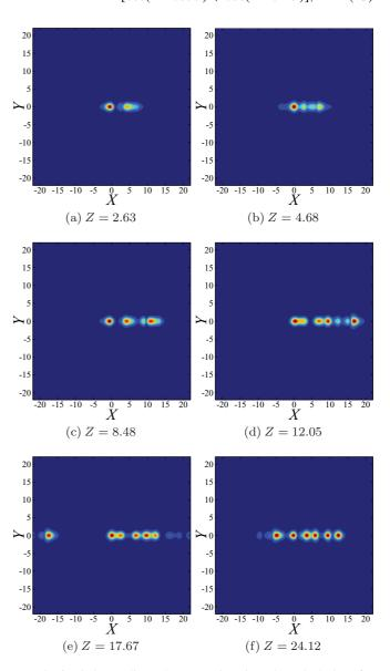
FIG. 6. (Color online) Same as in Figs. 3 and 5, but for  $k_0 = 1.694$ . In this case, the kicked soliton eventually creates an arrayed set of five solitons [in panel (f) the additional freely moving (sixth) soliton hits the array from the opposite direction, completing its round-trip in the system].
