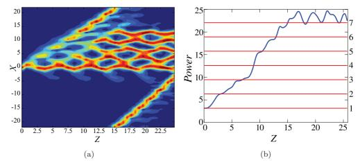
FIG. 11. (Color online) (a) Field amplitude |u(X,Z)| in the cross section Y = 0 and (b) evolution of the total power for the kick's strength  $k_0 = 1.693$  at  $\theta = 0$ , which leads to the establishment of the six-soliton pattern.
