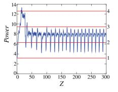
FIG. 4. (Color online) Evolution of the total power of the pattern in the case displayed in Fig. 3, with  $k_0 = 1.6878$  and  $\theta = 0$ . The horizontal lines show the powers for the sets of one to four quiescent fundamental solitons.
