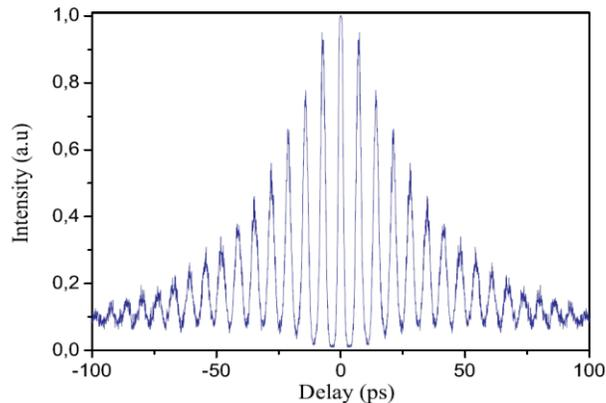
Fig. 3. Autocorrelation trace (experiment).
