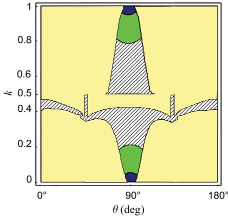
FIG. 4. (Color online) Variation of pulse energy in the  $(\theta, k)$  plane for  $L_2 = 19$  m and  $L_3 = 24$  m. In the blue (black) region, the energy is above 8 pJ; in the green (dark gray) region, the energy is between 2 and 8 pJ; and in the hatched region, the energy is below 2 pJ. In the yellow (light gray) region, either the pulses are unstable or their stability is not determined and continuous emission occurs.
