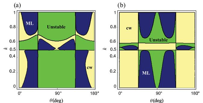
FIG. 2. (Color online) Stability diagram of the cw and ML solutions for (a)  $L_2 = 3$  m,  $L_3 = 2$  m and (b)  $L_2 = 7.5$  m,  $L_3 = 5$  m in the plane  $(\theta, k)$ . The yellow (light gray) region corresponds to stable cw and TXtable unstable ML operation, the blue (black) region corresponds to stable ML and unstable cw operation. The green (dark gray) corresponds to unstable cw and unstable ML operation.
