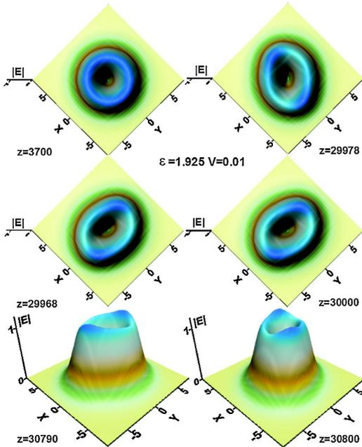
FIG. 3 (color online). The self-trapping of a stably rotating elliptic vortex. The configurations displayed at  $z = 29968$  and  $z = 30000$  correspond to the rotation of the ellipse by  $180^\circ$ . Images in the bottom row display the established shape of the elliptic vortex.
