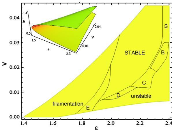
FIG. 1 (color online). Stability regions of vortex solitons in plane  $(\varepsilon, V)$  of the loss-modulation parameters. In this figure and below, other coefficients in Eq. (1) are  $\gamma = 0.29$ ,  $\mu = 1.4$ ,  $\nu = 0.4$ . The VA predicts the stability in the shaded area, and the corresponding amplitude displayed in the inset.
