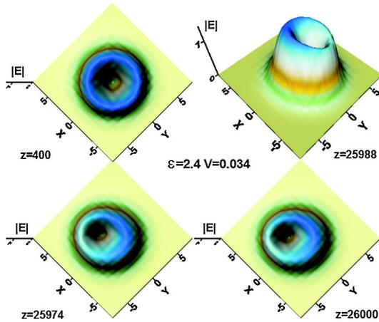
FIG. 6 (color online). A vortex breather formed from the VA-predicted input at  $z \approx 20$  and shown from above at  $z = 400$ , evolves into an elliptically-shaped “slanted volcano”, whose profile is displayed at  $z = 25988$ . It rotates with period  $Z \approx 26$  (the images shown at  $z = 25974$  and  $z = 26000$  are separated by the period).
