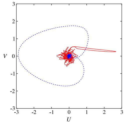
**Fig. 5.** Evolution of the polarization of the unstable CP FCP with both angular frequency and pulse length 1. Blue (dotted): initial CP pulse (at  $Z = 100$ ), red (solid): final linearly polarized pulse (at  $Z = 1300$ ).
