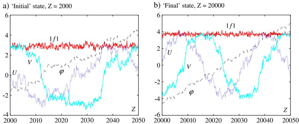
**Fig. 6.** One period of rotation of the slowly rotating LP half-cycle pulse resulting from the instability of the CP FCP with both angular frequency and pulse length 1, at the beginning of its evolution (a), and after long propagation (b). Red (thin solid): norm of the electric field  $|f|$ , blue (dotted): x-polarized component  $U$ , light blue (thick solid gray): y-polarized component  $V$ , black (dashed): phase  $\arctan(V/U)$ .
