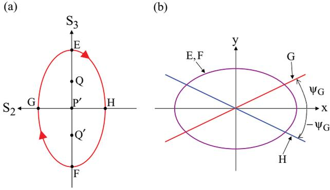
FIG. 10. (Color online) (a) Example of evolution around the point  $P'$  with points of interest. (b) Electric field polarization in the  $x$ - $y$  plane corresponding to the relevant points G (linear polarization), E (right-handed elliptical polarization), H (linear polarization), and F (left-handed elliptical polarization).
