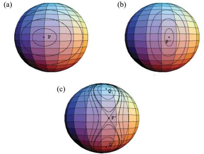
FIG. 11. (Color online) Evolution of the state of polarization in the Poincaré sphere. (a) Evolution around  $P$  when  $k > \Omega$ . (b) Evolution around  $P'$  when  $k > \Omega$ . (c) Case where  $k < \Omega$ . The double-loop curve is the boundary between  $Q$ - $Q'$  solutions and  $P$ - $P'$  solutions.
