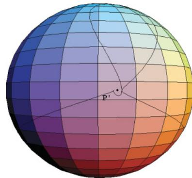
FIG. 13. (Color online) Evolution of the polarization state at the exit of the fiber in the Poincaré sphere as a function of  $\Omega$  for an incident polarization close to the unstable fast axis,  $\theta = 89^\circ$
