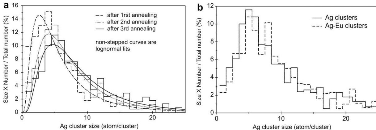
**Fig. 3.** Particle size distributions (a) after each annealing; lognormal fitting curves are drawn; and (b) comparison of Ag clusters distribution and Ag–Eu clusters distribution after the 3rd annealing.
