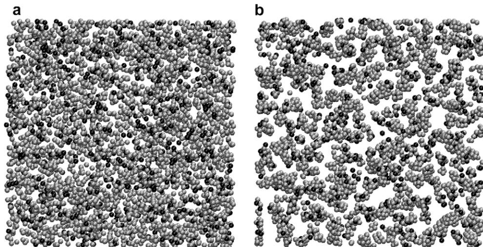
**Fig. 2.** Snapshots of the simulated microscopic structures.  $\text{Eu}^{+3}$  ions are in black and Ag atoms in grey. For clarity Si, Na and O are not drawn. (a) Snapshot before annealing, showing a homogeneous repartition of silver atoms and no cluster; and (b) after the annealing procedure pure Ag particles and Ag-Eu nanoalloys have been simulated.
