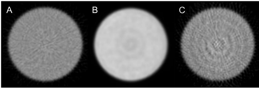
**Figure 1. Observed artefacts on images acquired on uniform phantom.** Display scale is [0; 100%]. A: no artefacts (site 9), B: LOR-RAMLA concentric ring artefacts (site 6), C: FBP concentric ring artefacts (site 4). doi:10.1371/journal.pone.0058152.g001
