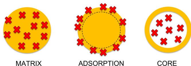
Fig. 2. Methods of siRNA complexation with delivery systems. The siRNA localization into nanocarriers differs according to structure and organization of the delivery system. siRNA can be incorporated into matrix structure and allows a global repartition in all volume of sphere (left). Second strategy consists to adsorb siRNA on surface of delivery systems in low depth (middle scheme). Last organization concerns shell/core structure observed for liposomes and some nanoparticles. In this case (right), siRNA is restrained in the core compartment of the delivery system.
