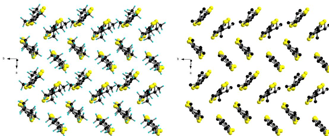
**Figure S5.** Crystalline packing of  $\kappa$ -[(*R,R*)-DM-BEDT-TTF]<sub>2</sub>ClO<sub>4</sub> in the conducting *ab* plane; H atoms (left), no H-atoms (right).
