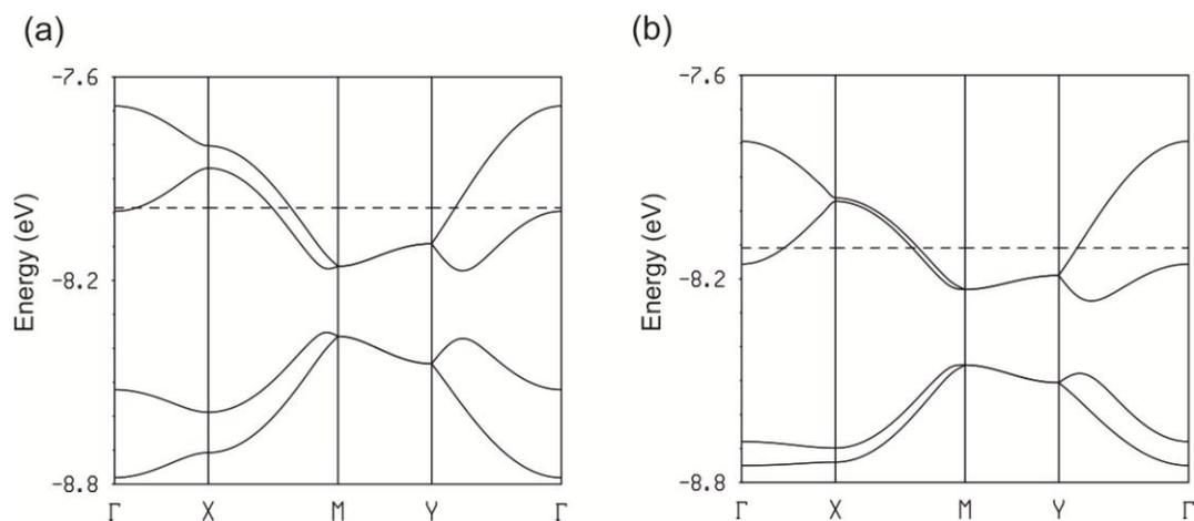
**Figure S6.** Extended Hückel band structure for the two donor layers of  $\kappa$ -[(*S,S*)-DM-BEDT-TTF]<sub>2</sub>ClO<sub>4</sub>: (a) layer type 1, and (b) layer type 2. The dashed line refers to the calculated Fermi level assuming two holes per layer.  $\Gamma = (0, 0)$ ,  $X = (a^*/2, 0)$ ,  $Y = (0, b^*/2)$ ,  $M = (a^*/2, b^*/2)$  and  $S = (-a^*/2, b^*/2)$ .
