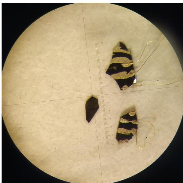
**Figure S21.** Millimeter size single crystalline plates of  $\kappa$ -[(*R,R*)-DM-BEDT-TTF]<sub>2</sub>ClO<sub>4</sub> for single crystal resistivity measurements.
