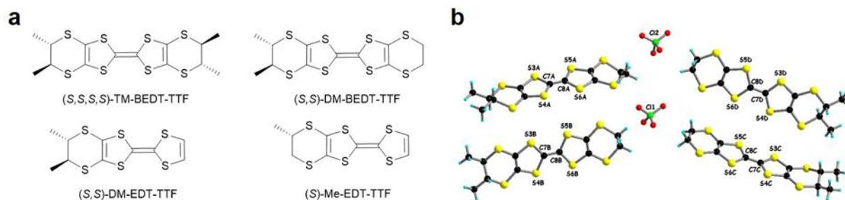
**Figure 1.** a) Enantiopure BEDT-TTF and EDT-TTF based donors including DM-BEDT-TTF, involved in this study. b) Crystalline structure of  $\kappa$ -[(*R,R*)-DM-BEDT-TTF]<sub>2</sub>ClO<sub>4</sub> highlighting the four independent donors and two anions in the asymmetric unit.
