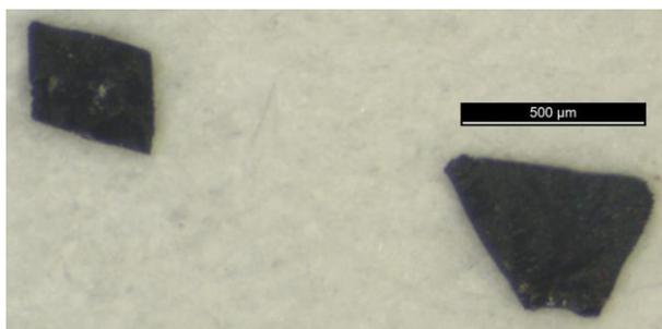
**Figure S17.** Picture of the black crystalline plates of  $\kappa$ -[(*S,S*)-DM-BEDT-TTF]<sub>2</sub>ClO<sub>4</sub>.
