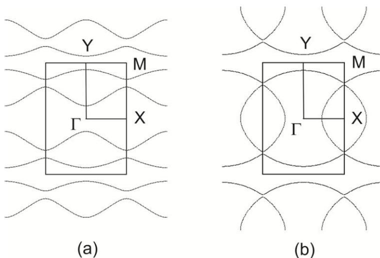
**Figure S9.** Extended Hückel Fermi surface for the two donor layers of  $\kappa$ -[(*S,S*)-DM-BEDT-TTF]<sub>2</sub>ClO<sub>4</sub> where the DFT hole transfer between the two layers is taken into account: (a) layer type 1, and (b) layer type 2.
