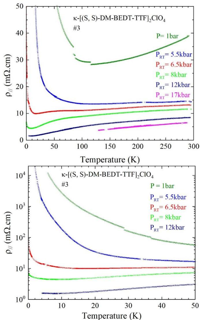
**Figure S12.** Temperature dependence of the in-plane electrical resistivity  $\rho_{||}(T)$  for a single crystal of  $\kappa$ -[(S,S)-DM-BEDT-TTF]<sub>2</sub>ClO<sub>4</sub> (#3) at different pressures, in the whole measured temperature range (top) and below 50 K (bottom). The resistivity of sample #3 under 17 kbar could not be measured below 130 K because of a contact to the ground of one of the wires in the feedthrough.
