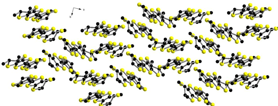
**Figure S3.** Crystalline packing of  $\kappa$ -[(*S,S*)-DM-BEDT-TTF]<sub>2</sub>ClO<sub>4</sub> in the conducting *ab* plane. ClO<sub>4</sub> anions have been omitted.
