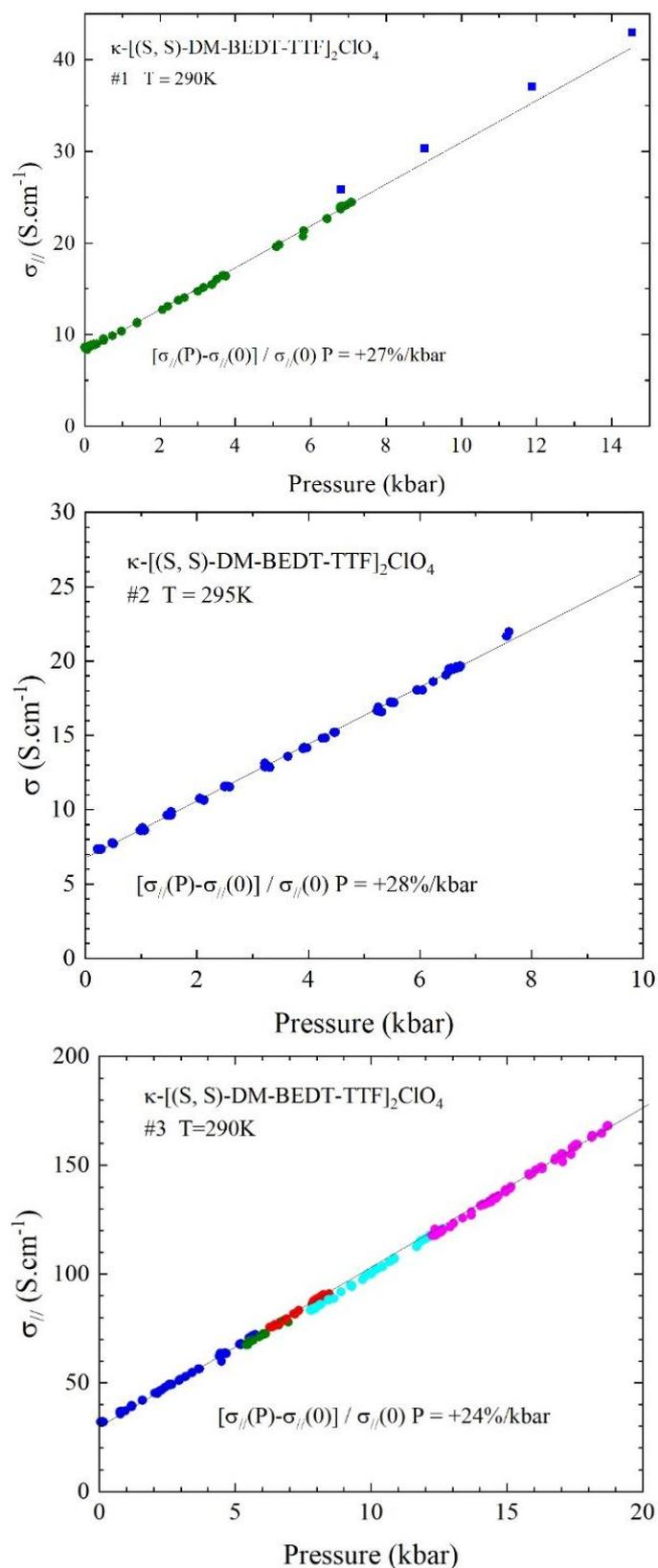
**Figure S14.** Pressure dependence of the in-plane electrical conductivity at room temperature for the three single crystals of  $\kappa$ -[(S,S)-DM-BEDT-TTF]<sub>2</sub>ClO<sub>4</sub> measured under pressure. The black line is the linear fit to the data.
