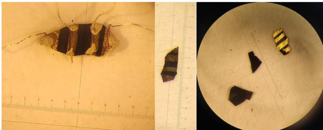
**Figure S20.** Millimeter size single crystalline plates of  $\kappa$ -[(*S,S*)-DM-BEDT-TTF]<sub>2</sub>ClO<sub>4</sub> for single crystal resistivity measurements.
