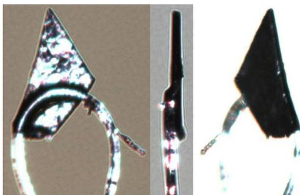
**Figure S18.** Different views of the measured single crystal of  $\kappa$ -[(*S,S*)-DM-BEDT-TTF]<sub>2</sub>ClO<sub>4</sub> mounted on a loop fiber in fomblin oil.
