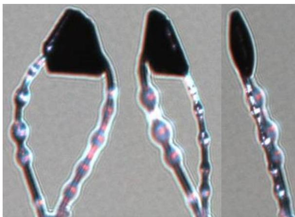
**Figure S19.** Different views of the measured single crystal of  $\kappa$ -[(*R,R*)-DM-BEDT-TTF]<sub>2</sub>ClO<sub>4</sub> mounted on a loop fiber in fomblin oil.
