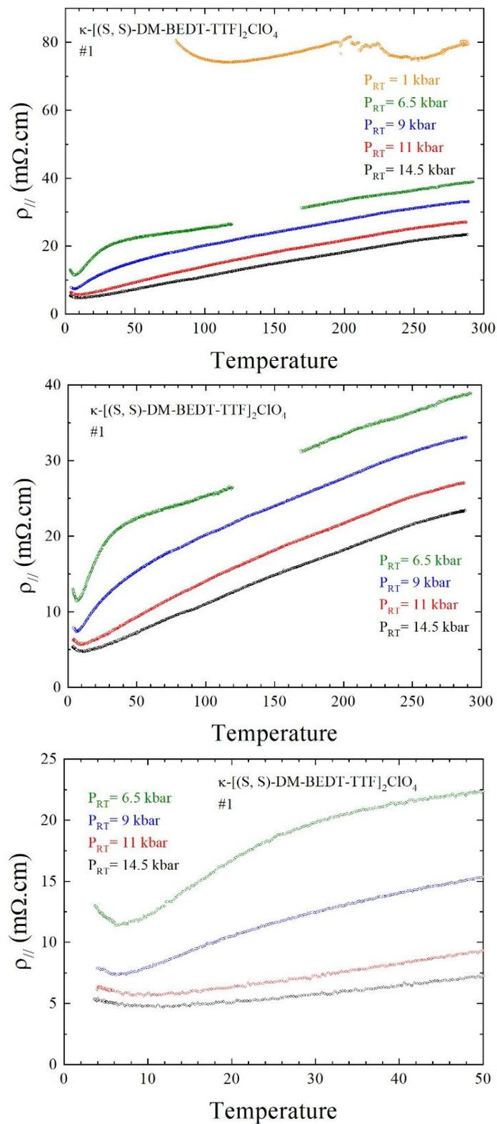
**Figure S10.** Temperature dependence of the in-plane electrical resistivity  $\rho_{||}(T)$  for a single crystal of  $\kappa$ -[(S,S)-DM-BEDT-TTF]<sub>2</sub>ClO<sub>4</sub> (#1) at different pressures, in the whole measured temperature range (two upper graphs) and below 50 K (bottom).
