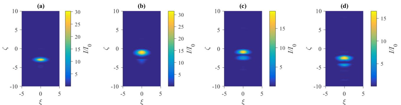
FIG. 4. The distribution of the energy density of the electric field,  $I(\xi, \nu_0, \zeta, \tau)$ , in the array of nanotubes at different values of dimensionless time  $\tau$ , when the laser pulse is reflected from the layer of increased electron concentration placed at  $\zeta = 0$ : (a)  $\tau = 0$ , (b)  $\tau = 3.0$ , (c)  $\tau = 6.0$ , (d)  $\tau = 9.0$ . The notation is the same as in Fig. 3.
