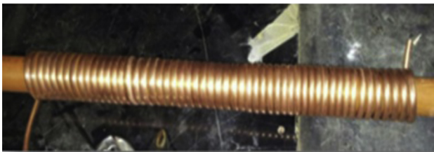
Fig. 4. Coiled heat exchanger used in the recovery system.
