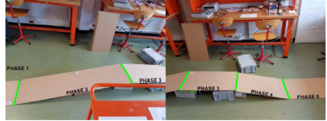
Fig. 4: Experimental setup : the expected trajectory is a straight line going through five phases with different slopes. The robot must move over the path at constant speed.
