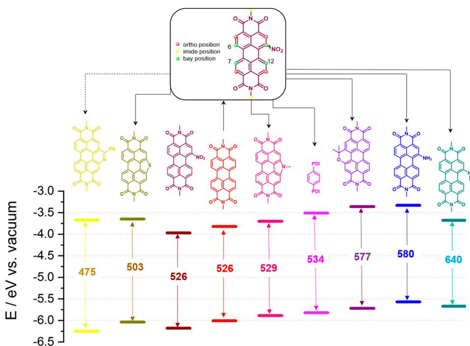
**Figure 1.** 1-NitroPDI, a key intermediate for reaching various bay-substituted-PDI structures with distinct photoredox properties. Frontier orbital energy (HOMO-LUMO) levels of PDIs. Wavelengths (nm) of maximal absorption of light are shown. The data were collected from references [30–35].
