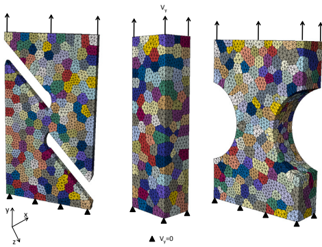
Fig. 4. Geometrical models and boundary conditions for tensile and shear tests
