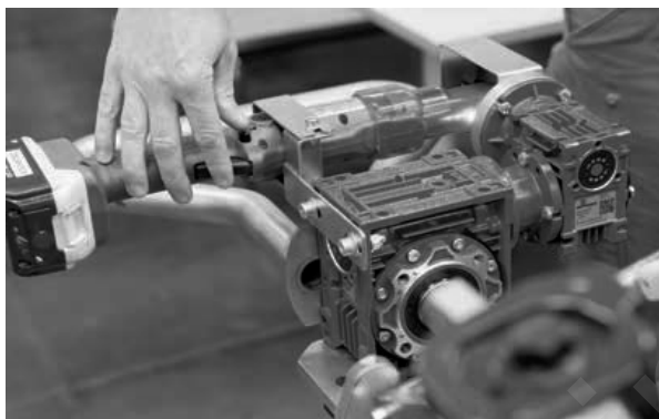
Figure 7. a) Manually turning the Selective Catalyst Reduction (SCR) wagon handle (repeated action). b) A screwdriver replaced the manual turning handle, which eliminated repeated actions.
