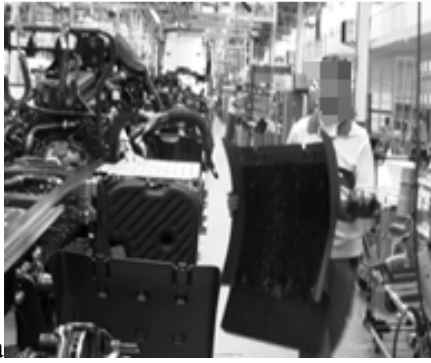
Figure 6. a. Lifting and carrying of rear mudguards (15kg) manually, major risk factor for low back pain; b) new lifting tool used for lifting and carrying mudguards
