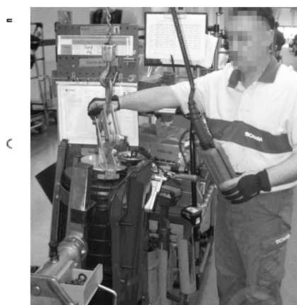
Figure 5. A new gripping tool for lifting air filter eliminated the risk of low back pain due to lifting a heavy object
