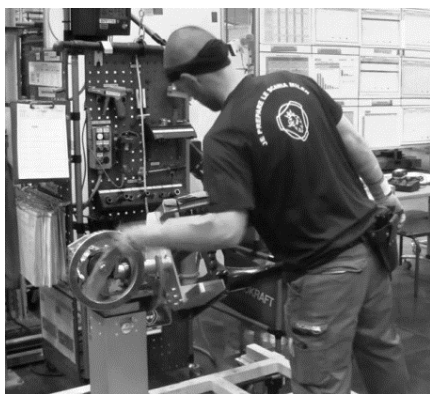
Figure 7. a) Manually turning the Selective Catalyst Reduction (SCR) wagon handle (repeated action). b) A screwdriver replaced the manual turning handle, which eliminated repeated actions.
