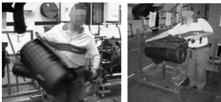
Figure 4. Lifting and carrying air filter (12-16 kg based on truck variants) caused low back pain and awkward posture
