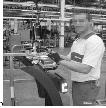
Figure 6. a. Lifting and carrying of rear mudguards (15kg) manually, major risk factor for low back pain; b) new lifting tool used for lifting and carrying mudguards
