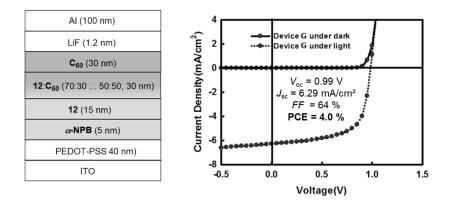
Figure 10: Vacuum-processed BHJ OSC based on **DA-10** and current density *vs* voltage curves under AM 1.5 white light illumination at 100 mW/cm<sup>2</sup>. Adapted from ref.105.
