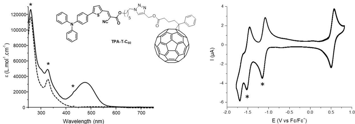
**Figure 13:** Structure of **TPA-T-C<sub>60</sub>**, UV-vis spectra of **TPA-T-C<sub>60</sub>** (solid line) and PC<sub>61</sub>BM (dashed line) in CH<sub>2</sub>Cl<sub>2</sub> and CV of **TPA-T-C<sub>60</sub>** in 0.1 M Bu<sub>4</sub>NPF<sub>6</sub>/CH<sub>2</sub>Cl<sub>2</sub>, Pt working electrode, scan rate 100 mV/s. The stars highlight the electrochemical and optical signatures of the fullerene moiety of **TPA-T-C<sub>60</sub>**. Adapted from ref. 121.
