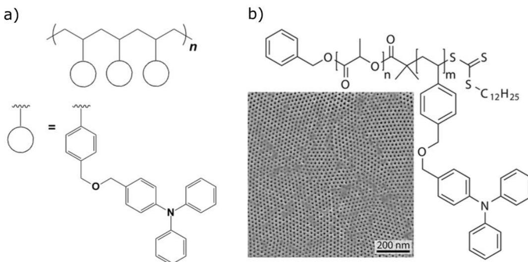
**Figure 4:** Chemical structures of **a)** PSTPA (ref. 44) and **b)** Chemical structure of PSTPA-*b*-PLA diblock copolymer, consisting of a triphenylamine side group polymer block and a poly(D,L-lactide) block (PLA); SEM image of the surface of an electroactive PSTPA porous template structure after PLA removal. Figure adapted from ref.36.
