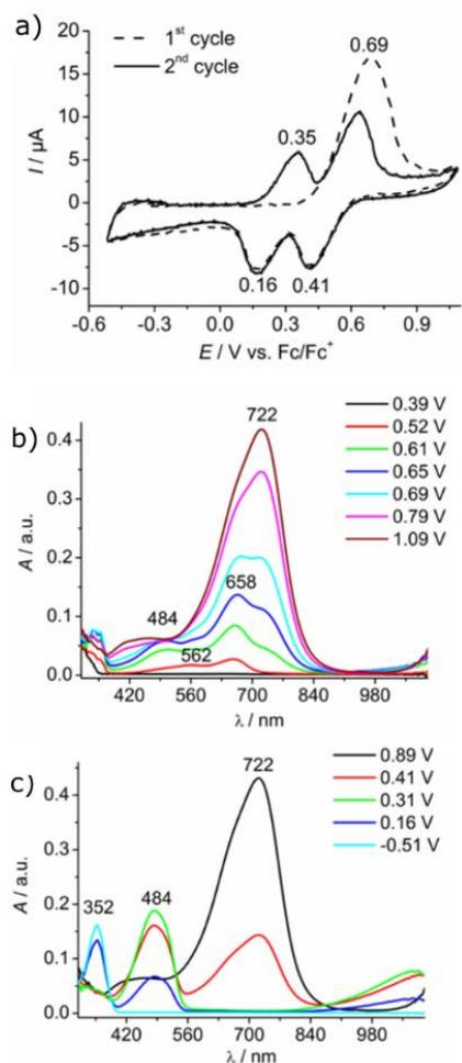
**Figure 2:** TPA oxidation in thin layer cell (0.1M TBAPF<sub>6</sub>/CH<sub>2</sub>Cl<sub>2</sub>; scan rate 20 mV/s), in situ spectroelectrochemical measurements. **a)** CV measurement with *in situ* UV-vis absorption spectra recorded for the first voltammetric cycle during **b)** charging and **c)** discharging. Figures adapted from ref. 34.
