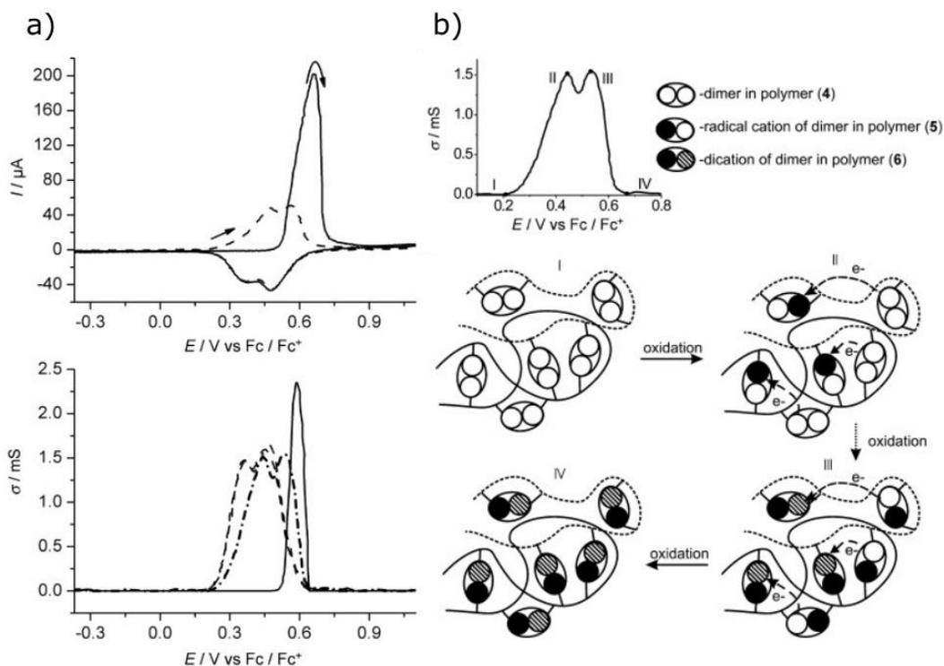
**Figure 5:** a) CV and *in situ* conductance measurements for PSTPA polymer films (MeCN/TBAPF<sub>6</sub> 0.1 M; scan rate 20 mV/s), first and second cycle and corresponding *in situ* conductance pattern measured simultaneously. b) Explanation of the respective redox species and conductivity profile in crosslinked PSTPA polymer films. Figures adapted from ref. 44.
