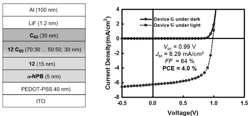
**Figure 10:** Vacuum-processed BHJ OSC based on **DA-10** and current density vs voltage curves under AM 1.5 white light illumination at 100 mW/cm<sup>2</sup>. Adapted from ref.105.
