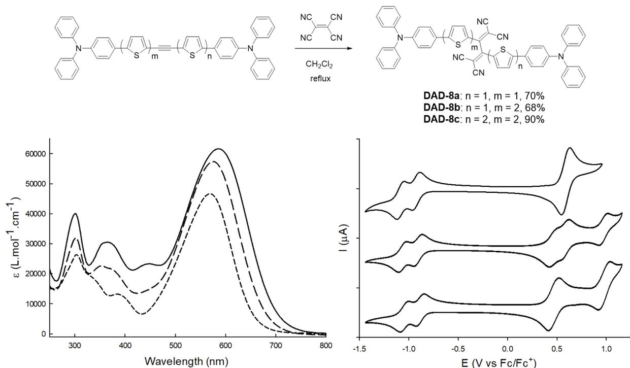
**Figure 8:** Synthesis of **DAD-8**. Left: Absorption spectra of **DAD-8a** (solid line), **DAD-8b** (long dashed line) and **DAD-8c** (short dashed line) in  $\text{CH}_2\text{Cl}_2$ . Right: CVs of **DAD-8a** (top), **DAD-8b** (middle) and **DAD-8c** (bottom) 0.5 mM in 0.1 M  $\text{Bu}_4\text{NPF}_6/\text{CH}_2\text{Cl}_2$ , Pt working electrode, scan rate 100 mV/s. Adapted from ref. 85.
