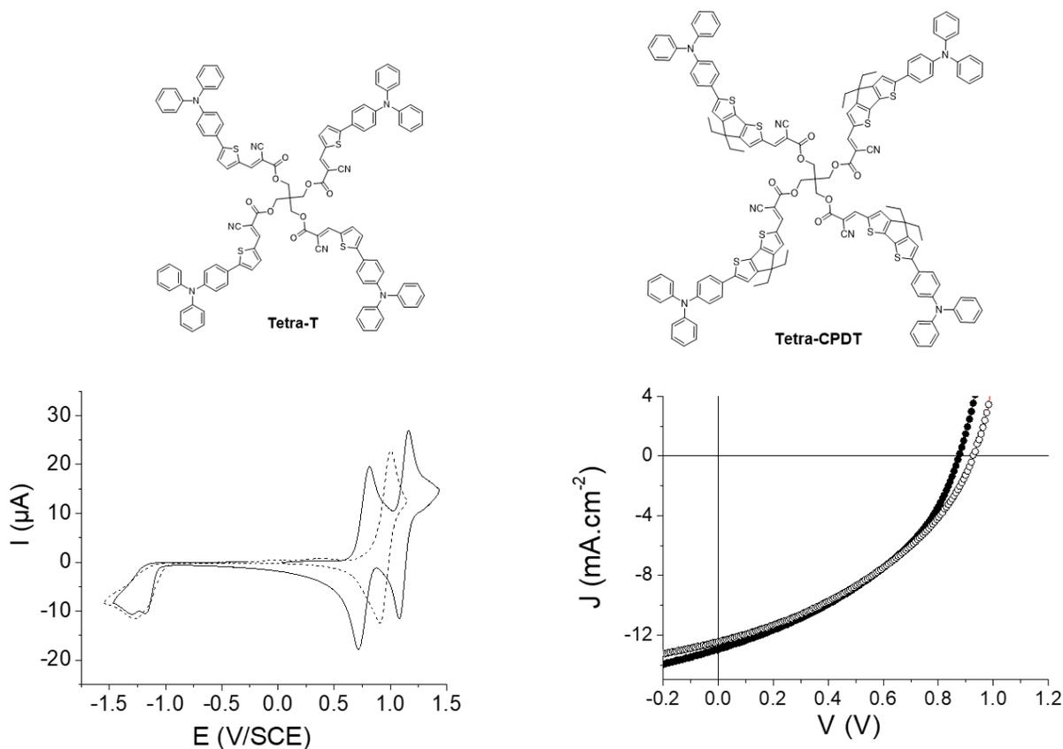
**Figure 12:** CV of **Tetra-T** (dashed line) and **Tetra-CPDT** (solid line) 0.5 mM in 0.1 M  $\text{Bu}_4\text{NPF}_6/\text{CH}_2\text{Cl}_2$ , Pt working electrode, scan rate 100 mV/s and current density vs voltage curves of BHJ OSCs prepared from **Tetra-T** (white circles) and **Tetra-CPDT** (black circles) under AM 1.5 white light illumination at  $100 \text{ mW/cm}^2$ . Adapted from reference 116 by permission of *The Royal Society of Chemistry*.
