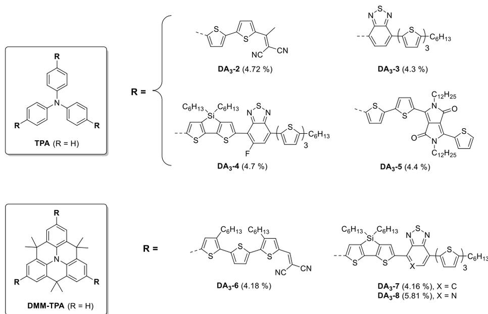
**Scheme 2:** Representative examples of TPA-based DA<sub>3</sub> push-pull donors and *PCE* values of PC<sub>71</sub>BM-based BHJ single junction OSCs.
