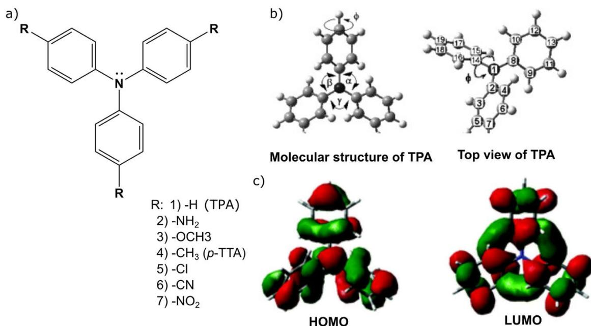
**Figure 1:** a) Chemical structures of TPA and *para*-substituted derivatives. b) Propeller like structure of TPA with three tilted phenyl rings. Adapted from ref. 25. c) DFT calculated HOMO and LUMO for TPA. Figure adapted from ref. 4.
