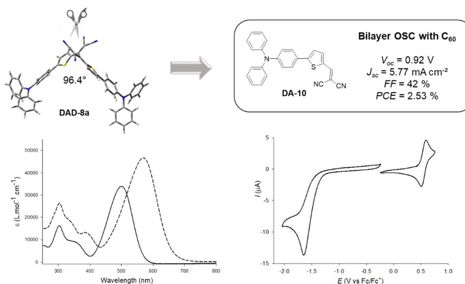
**Figure 9:** DFT-optimized geometry of **DAD-8a** (Gaussian 09 B3LYP/6-31G(d,p) level) and structure of **DA-10** corresponding to half of **DAD-8a** and related photovoltaic performance (Top). Absorption spectra of **DAD-8a** (dashed line) and **DA-10** (solid line) in CH<sub>2</sub>Cl<sub>2</sub> (bottom left) and CV of **DA-10** 0.5 mM in 0.1 M Bu<sub>4</sub>NPF<sub>6</sub>/CH<sub>2</sub>Cl<sub>2</sub>, Pt working electrode, scan rate 100 mV/s (bottom right).
