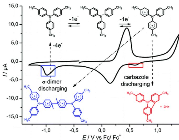
**Figure 3:** CV in thin layer cell of tri-*p*-tolylamine in TBAPF<sub>6</sub>/CH<sub>2</sub>Cl<sub>2</sub> 0.1 M, scan rate 20 mV/s, with peak assignment for the products of the reversible and irreversible follow up reactions from ref. 34.
