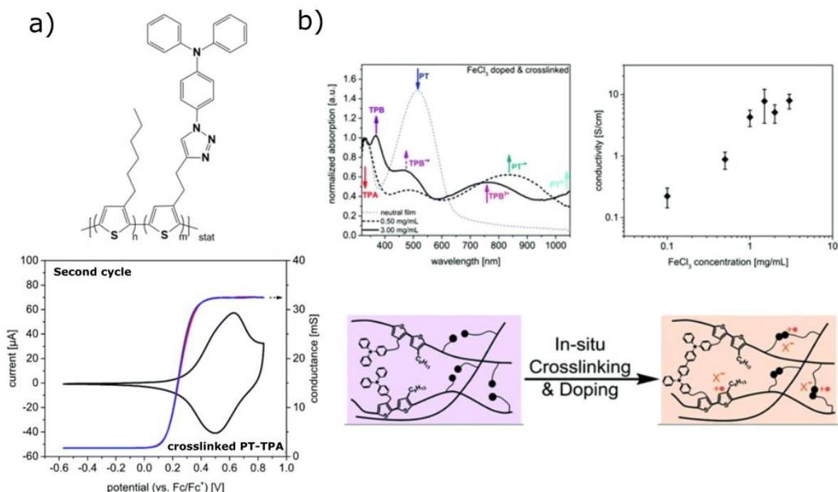
**Figure 6:** a) CV and *in situ* conductance measurement for a crosslinked PT-TPA thin film b) Absorption spectra and conductivity measurements of crosslinked PT-TPA for different dopant solution ( $\text{FeCl}_3/\text{CHCl}_3$ ) concentrations. Figures adapted from ref. 57.
