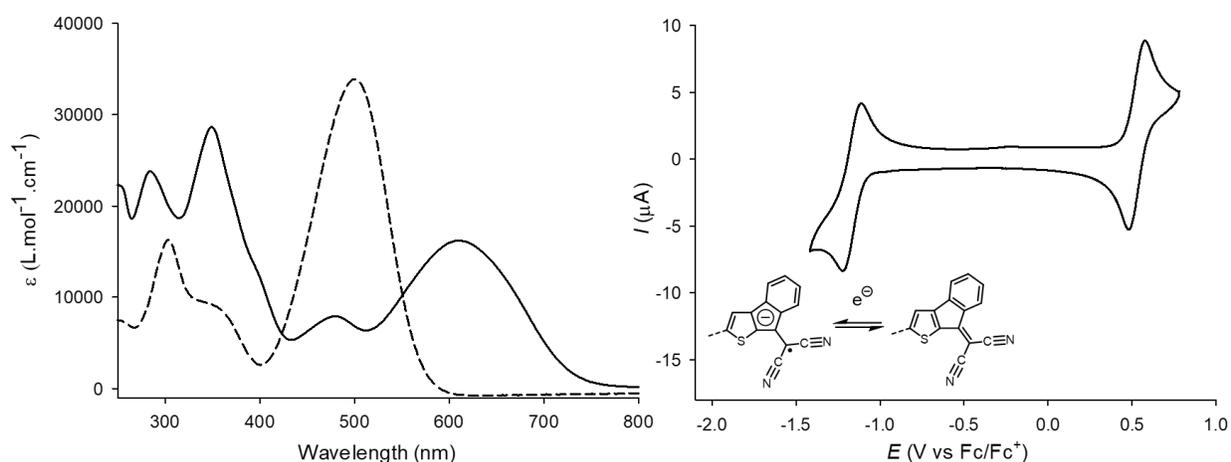
**Figure 11:** Absorption spectra of **DA-10** (dashed line) and **DA-13** (solid line) in CH<sub>2</sub>Cl<sub>2</sub> (Left). CV of **DA-13** 1 mM in 0.1 M Bu<sub>4</sub>NPF<sub>6</sub>/CH<sub>2</sub>Cl<sub>2</sub>, Pt working electrode, scan rate 100 mV/s and generation of a cyclopentadienyl radical anion upon electrochemical reduction (Right).
