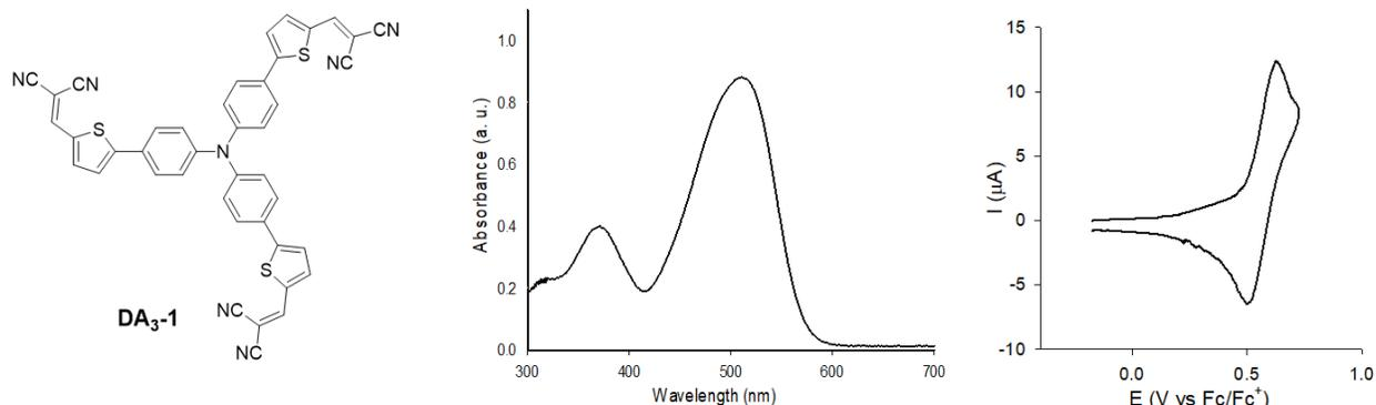
**Figure 7:** Structure of **DA<sub>3</sub>-1** (left), UV-vis spectrum in CH<sub>2</sub>Cl<sub>2</sub> (middle) and CV in 0.1 M Bu<sub>4</sub>NPF<sub>6</sub>/CH<sub>2</sub>Cl<sub>2</sub> (right), Pt counter and working electrodes, scan rate 100 mV/s. Adapted from ref 60.
