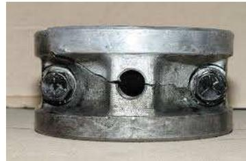
Fig.1. Failure of circular cylindrical bearing
